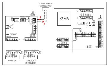
Figure 31 – Remove 2-10VDC motor control signal
