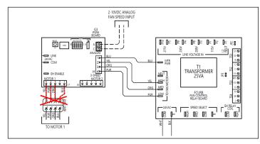
Figure 50 – Remove Motor Signal Wires
