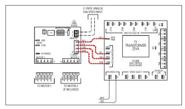
Figure 23 - Remove low voltage signal wires to motor(s)
