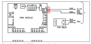
Figure 17 - Remove 2-10VDC motor control signal
