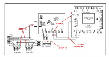
Figure 61 – Sync PWM Electrical Connections
