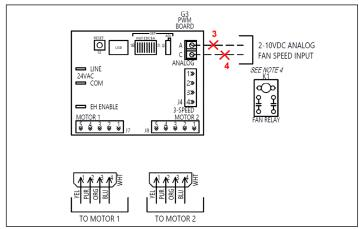
Figure 45 - Remove 2-10VDC motor control signal
