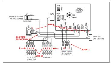
Figure 19 - Sync PWM Electrical Connections
