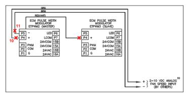
Figure 10 - Remove 2-10VDC motor control signal
