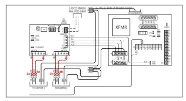
Figure 72 – Remove Motor Signal Wires
