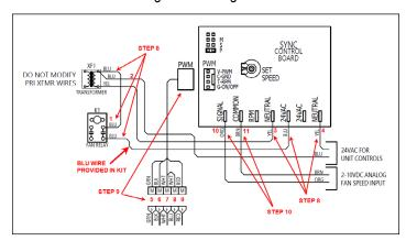
Figure 6 – Sync PWM Electrical Connections
