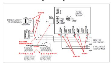
Figure 12 – Sync PWM Electrical Connections
