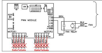
Figure 15 - Remove Motor Signal Wires
