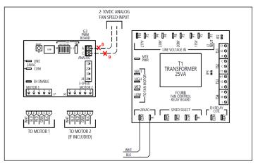
Figure 24 – Remove 2-10VDC motor control signal
