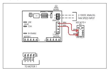
Figure 37 - Remove low voltage signal wires to motor(s)
