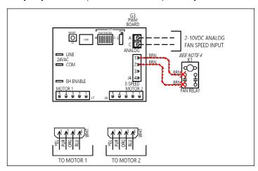
Figure 44 - Remove low voltage signal wires to motor(s)
