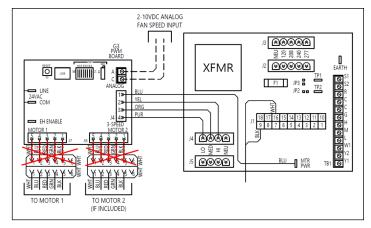
Figure 29 – Remove Motor Signal Wires
