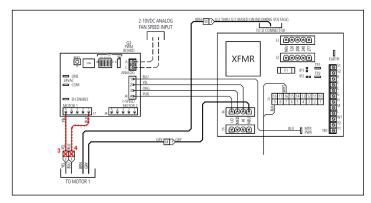
Figure 64 - Remove Motor Signal Wires
