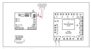
Figure 52 - Remove 2-10VDC motor control signal
