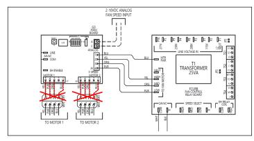
Figure 57 – Remove Motor Signal Wires
