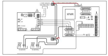
Figure 73 - Remove Motor Signal Wires
