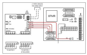
Figure 30 - Remove low voltage signal wires to motor(s)
