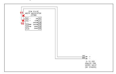
Figure 3 - Remove Motor Signal Wires
