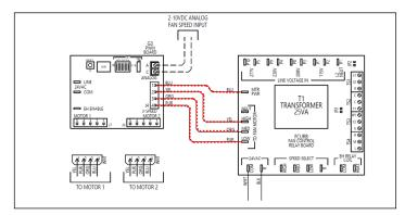
Figure 58 - Remove low voltage signal wires to motor(s)
