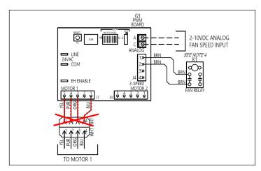
Figure 36 – Remove Motor Signal Wires
