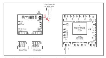
Figure 59 - Remove 2-10VDC motor control signal
