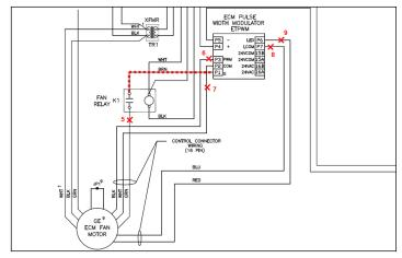
Figure 3 - Remove Motor Signal Wires
