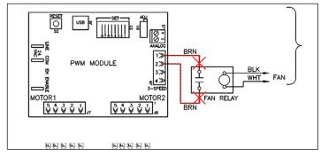
Figure 16 - Remove low voltage signal wires to motor(s)
