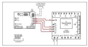
Figure 57 - Remove low voltage signal wires to motor(s)
