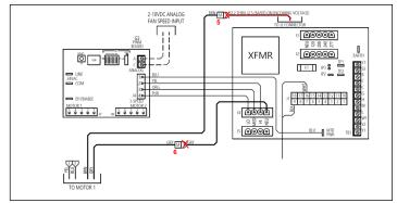
Figure 65 - Remove Motor Signal Wires
