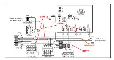
Figure 47 – Sync PWM Electrical Connections
