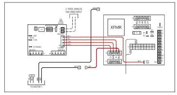
Figure 66 - Remove low voltage signal wires to motor(s)
