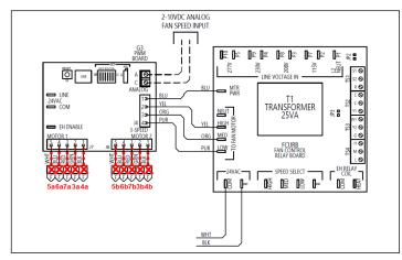
Figure 22 - Remove Motor Signal Wires
