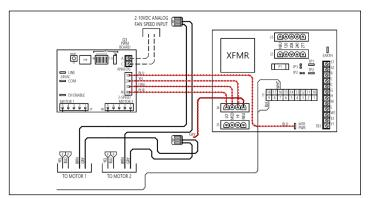
Figure 74 - Remove low voltage signal wires to motor(s)
