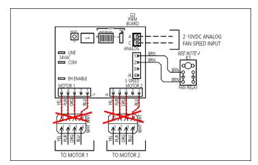
Figure 43 – Remove Motor Signal Wires
