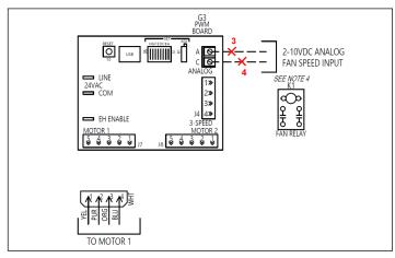
Figure 38 - Remove 2-10VDC motor control signal
