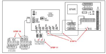
Figure 33 - Sync PWM Electrical Connections
