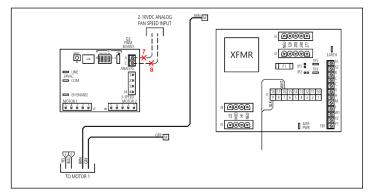
Figure 67 - Remove 2-10VDC motor control signal
