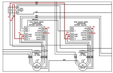
Figure 9 - Remove low voltage signal wires to motor
